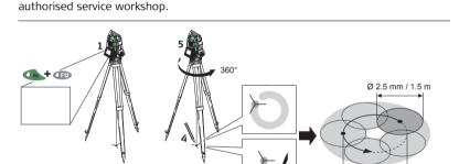
The laser plummet is located in the vertical axis of the instrument. Under normal conditions of use, the laser plummet does not need adjusting. If an adjustment is necessary due to external influences, return the instrument to any Leica Geosystems
