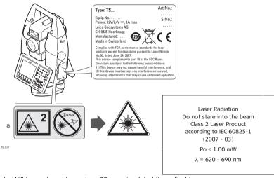
a) Will be replaced by a class 3R warning label if applicable
